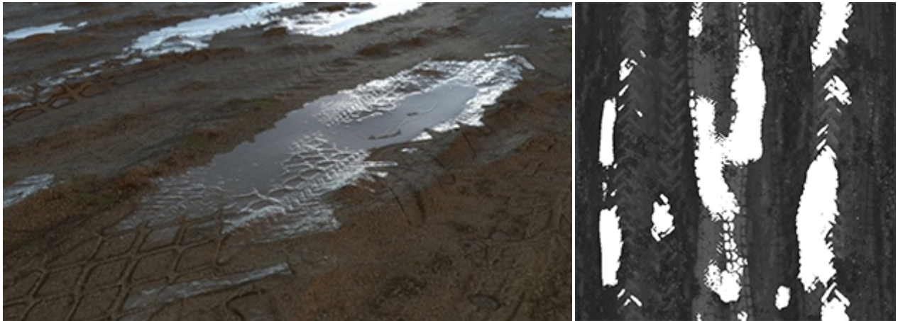
Rollover image (left). Puddles are created with a glossy texture map connected to coat_normal via bump shader (right).
