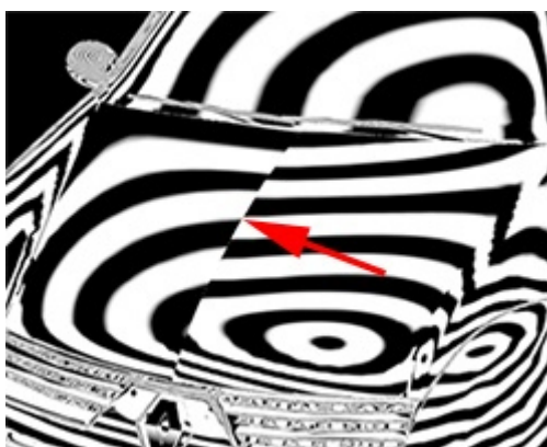
reflection_lines reveals continuity error in hood of car geo (rollover image)
